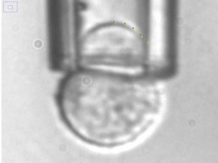
Figure 9: Discrete points used to capture the right half of cell membrane projection inside micropipette. These control points are later imported into Matlab to generate a curve that could be represented by a polynomial function.
